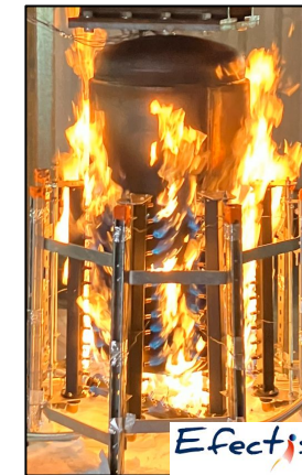
S235 steel tank subjected to fire (Efectis test)
