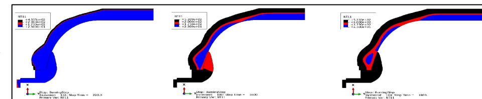
Evolution of the melting front in the composite tank
