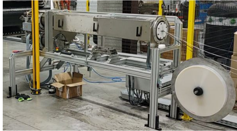
Preheating the tape into melt
