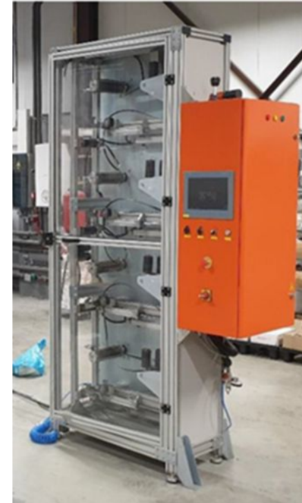
UD tape bobbin tensioning device Detailed tension control for every bobbin
