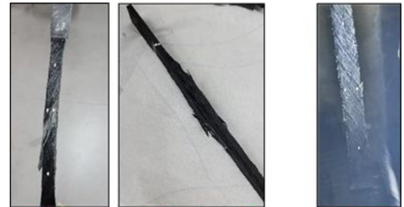
Tensile testing on 45° sample at 25°C
