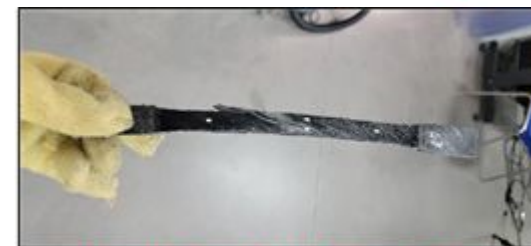
Elongated sample (45°) after tensile testing
